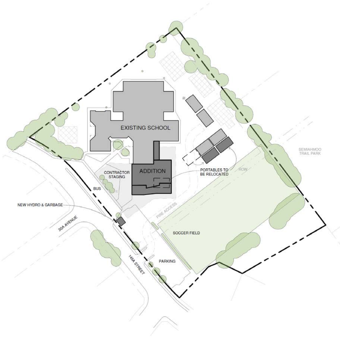
Site Plan During Construction
